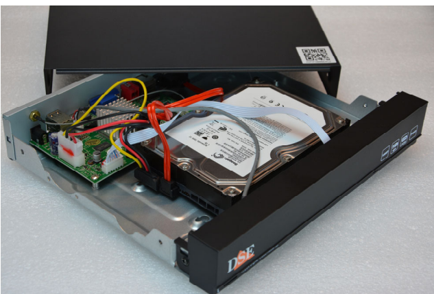
Secure the hard disk with the 4 screws provided screw in from underneath the VCR
