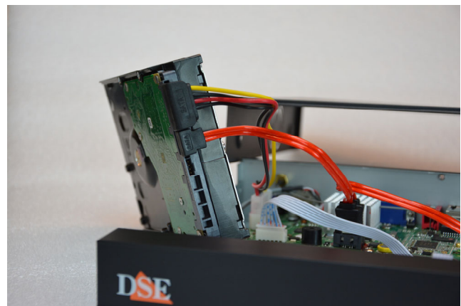
Connect the hard disk with the two power and data cables found inside
