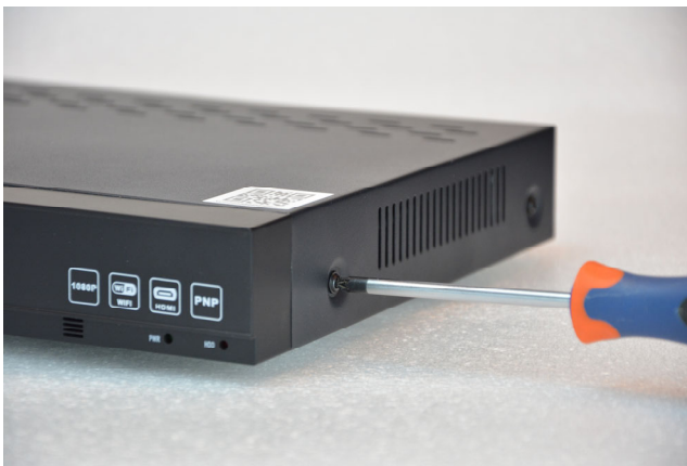
Remove the cover by unscrewing the 5 screws
