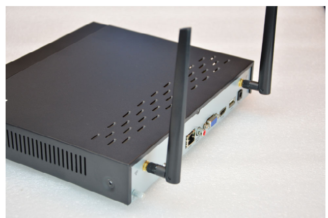
Close the lid and screw the 2 antennas onto back of the appliance
